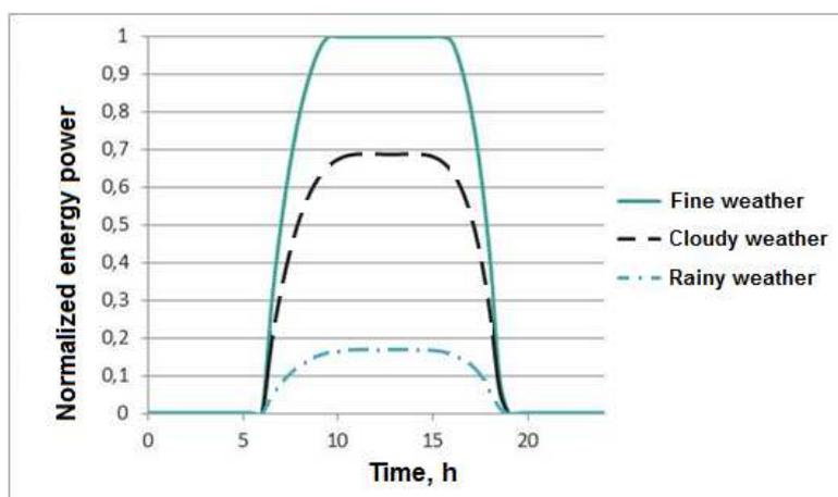
Fig. 3 Relative photovoltaics power vs hours according to weather conditions
