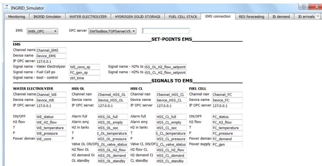
Fig. 2 Connection panel between the INGRID simulation tool and the EMS
