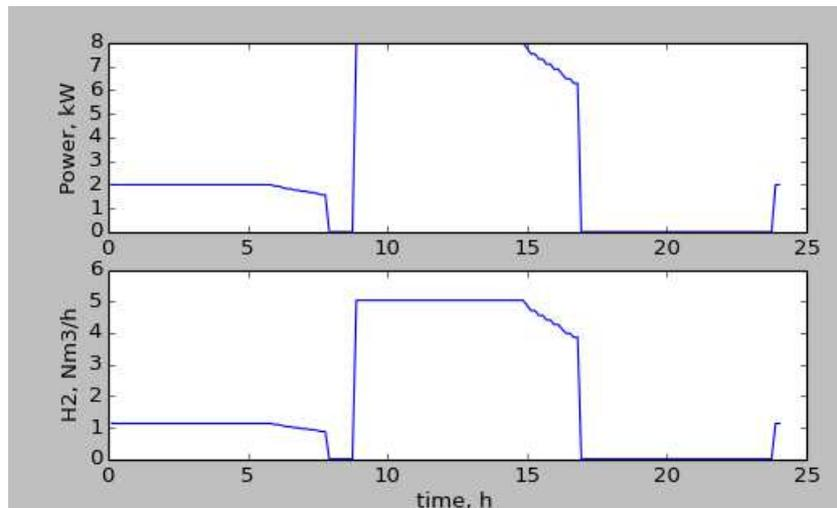
Fig. 8 Fuel cell dynamics for the required electric vehicle power demand.
