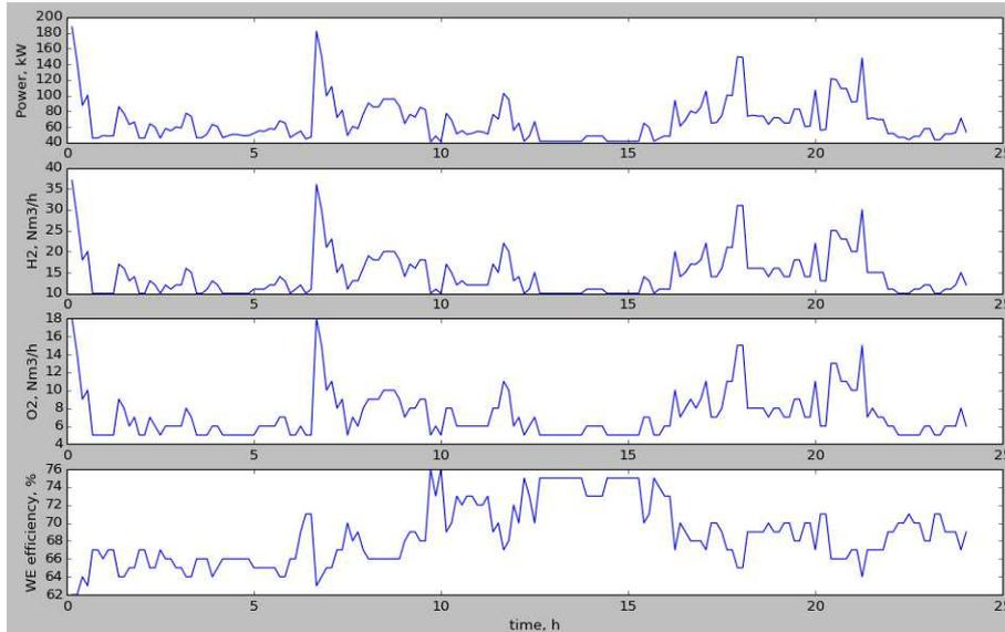
Fig. 6 The water electrolyser behavior according to the EMS logic.
