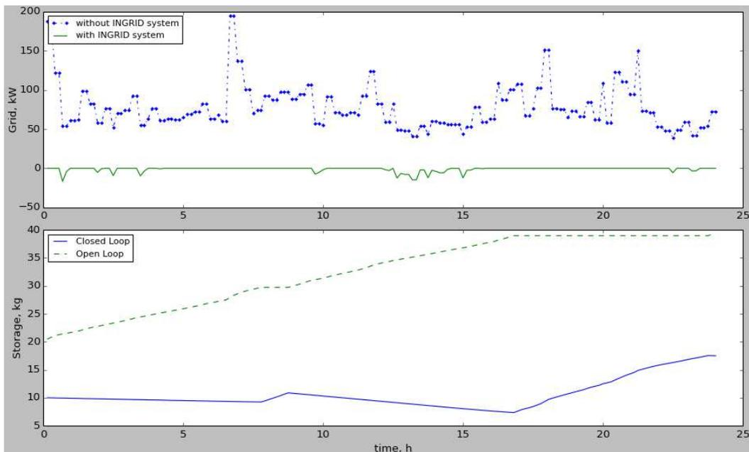
Fig. 5 Surplus power production with and without INGRID system and hydrogen storage in closed and open loop.
